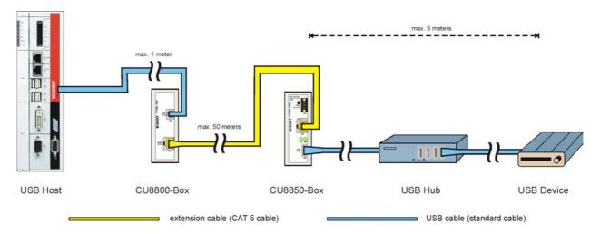
The USB hub is connected after the extension. The maximal distance is also 56 meters: 1 meter of cable from USB host to the USB extension box CU8800; up to 50 meters extension cable; 5 meters from extension box to the USB device via the USB hub.
