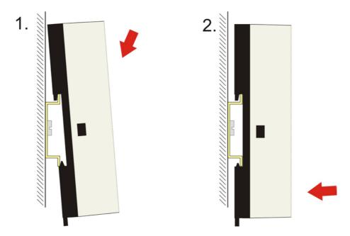
To release the CU8800-0010 from the mounting rail:
