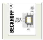
The USB-Extender-Tx does not need any additional power supply. The power supply (5 V DC) is realized by the USB connector. The LED **P10** lights green when power supply is connected.
