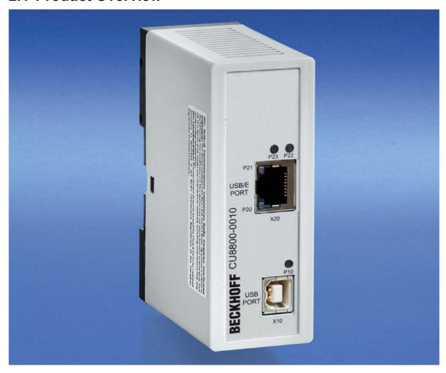
The Beckhoff CU8800-0010 USB-Extender-Tx allows to extend the limits of USB cable length. Standard USB cable are specified for cable length up to 5 meters. For some industrial applications there is need for longer distances. This box can extend the distance up to 50 meters. This box sends the USB signals from input port to the receiver box CU8850 or CU8860. Other outstanding features are:
