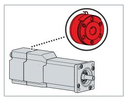
A holding brake blocks the rotor in the de-energized state. The holding brake increases the motor length and the rotor moment of inertia. The holding brake cannot be retrofitted and is mounted on the B bearing side of the servo drive.
