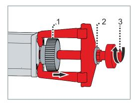
Use only backlash-free and friction-locked collets, gear pullers or suitable couplings to dismount the output elements.
