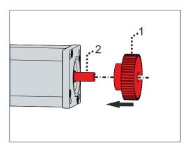
▶ Place output element [1] centered and straight on the shaft [2]
