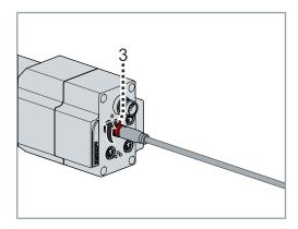
► Screw thread [3] into the socket
