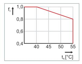
Derating may be necessary at high ambient temperature or when operating at a great height above sea level. In addition, some servo drives may experience power reductions depending on the feedback system installed or the holding brake [+]. The reduction affects the standstill current and the standstill torque.
