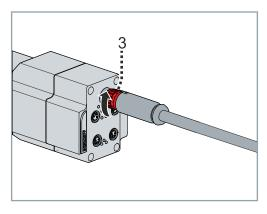
► Screw thread [3] into the socket
