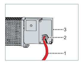
► Feed a sufficiently dimensioned cable 1 through the clamping device 2 into the terminal box 3
