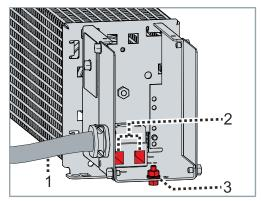
► Connect the cable 1 to the connections 2 and the earthing point 3
