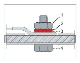
► Earth the surface as shown in the illustration with nut 1, spring washer 2, washer 3 and bolt 4
